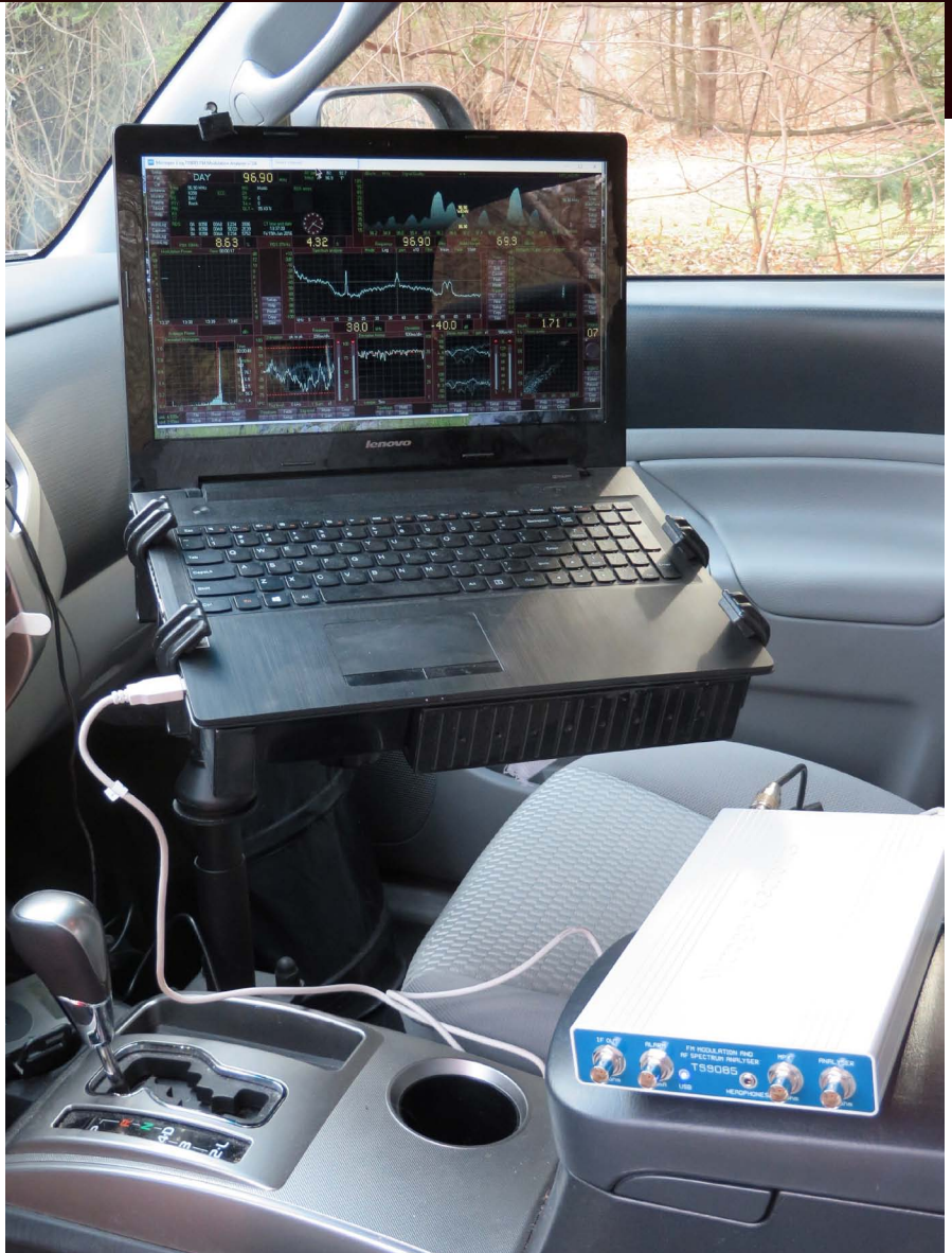
Fig. 1: Tools of the trade — typical equipment setup for mobile FM field strength measurements in the cab of a truck.
