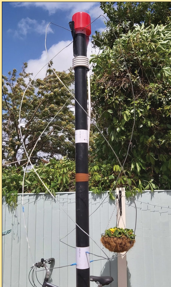
Rob Bale's smart looking QFH antenna, constructed in an evening from 'bits and bobs'
