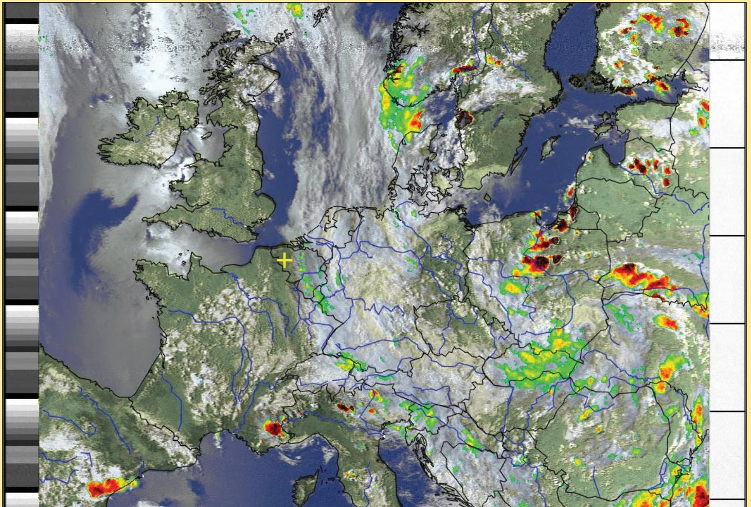
André T'Kindt J010TR submitted this NOAA 19 APT image acquired at 17:24 UT on May 21, 2019. It was captured using a turnstile antenna and preamp and processed in WXtolg using its *HVCT with precipitation* mode.
