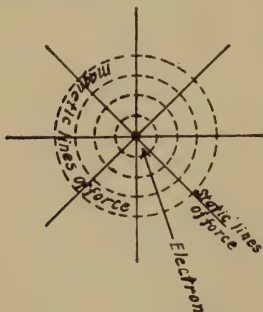
FIG. 14. Electron in Motion Produces Magnetic Lines of Force.
