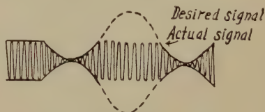
FIG. 153. An Improperly Modulated Wave.
