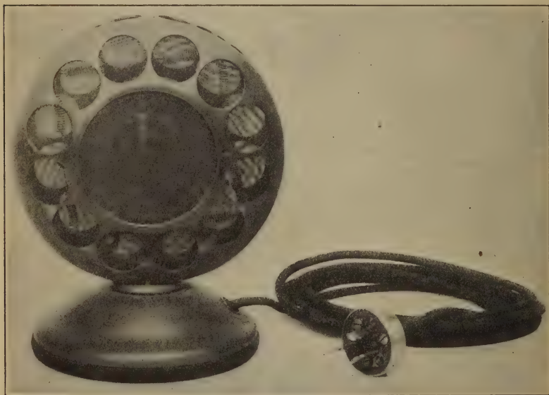
FIG. 149. Western Electric No. 373-W Transmitter (Double-Button).
