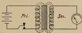
FIG. 16. Production of Current in a Secondary Circuit by Electro-Magnetic Induction.
