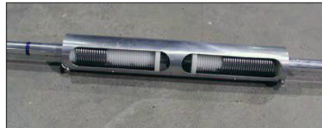
Figure 1 — Cutaway view shows a two-coil trap. The coils and tube capacitance form a resonant circuit, and the 2-inch outer tube is part of an element (usually for 15 meters).
