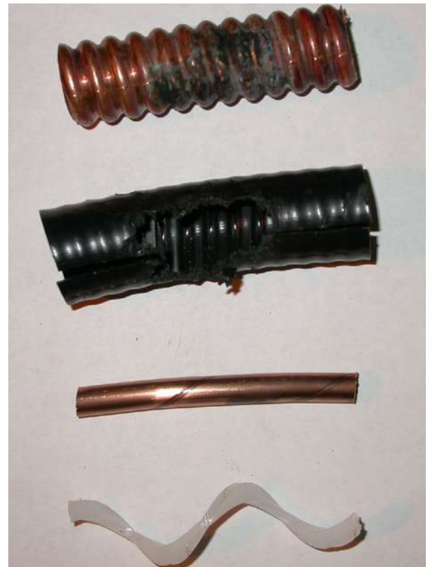
Right These damaged components are an example of the "outside in" sort of burn that can occur when lines pass too close or touch other coax or tower members.
