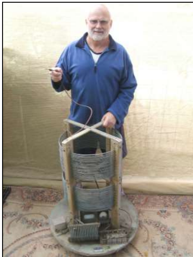
Doc, VK5BUG – "That's a coil!" for a duo-band 170ft Inverted-L 3-wire capacity hat & 60 dripper irrigated radials
