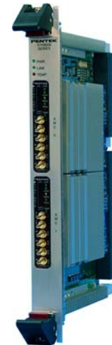
Model 58761 6U VPX dual density
