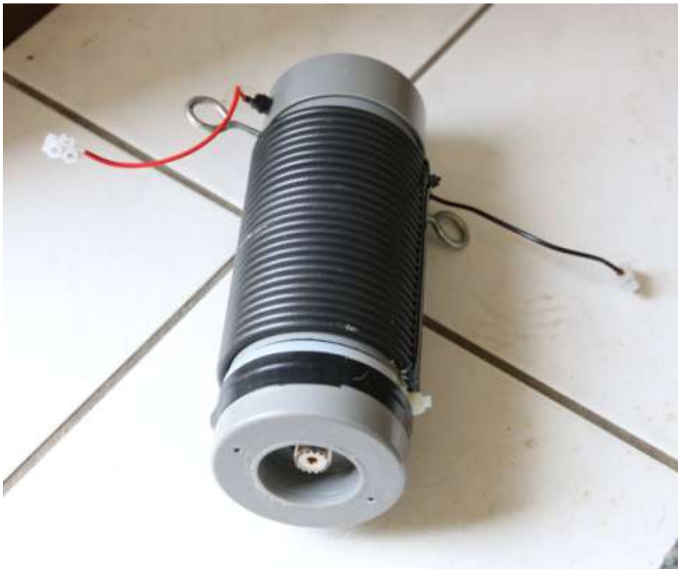
Picture 3 - Ugly balun - Red and black wires connect the dipole with the inner and outer conductors of the coax
