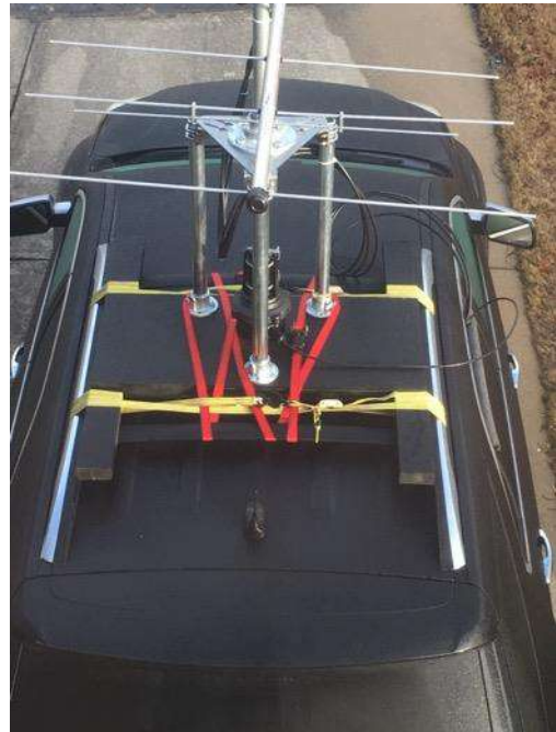
Figure 63 - Rooftop mounting system
