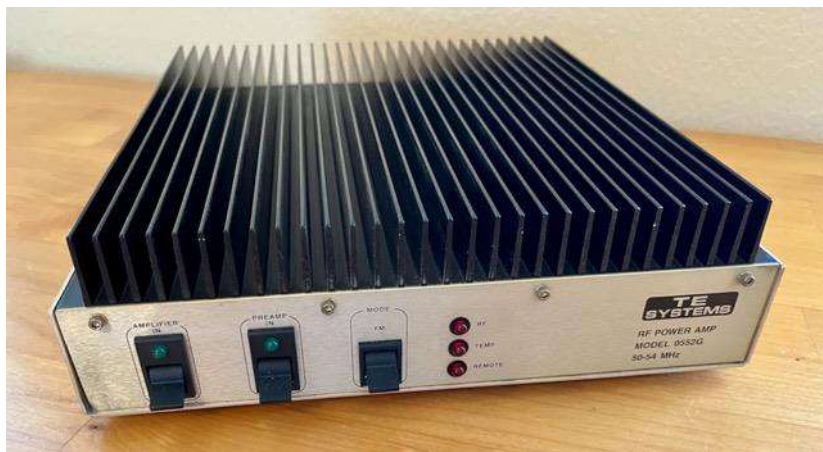
Figure 14 - TE Systems 375 Watt Six Meter Amplifier
