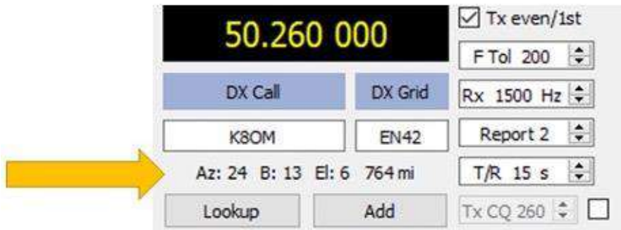
Figure 52 - Recommended Elevation and Azimuth
