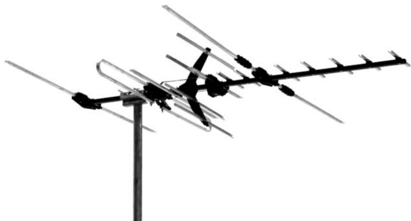
Figure 5.14 Conventional outdoor TV antenna
