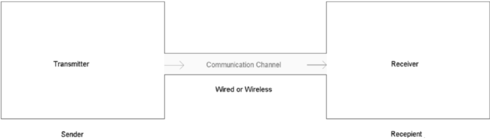
Figure 2.1 Block diagram of a basic communication system
