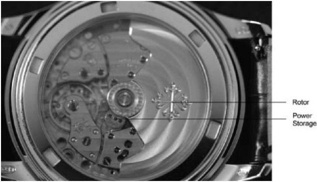
Figure 9.6 Automatic winding movement mechanism
