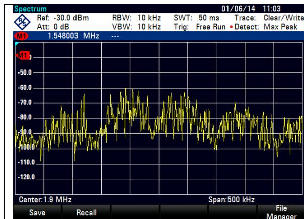
Figure 2: Peak measurement at an amateur radio station 4,5 km from Wind Farm 1
