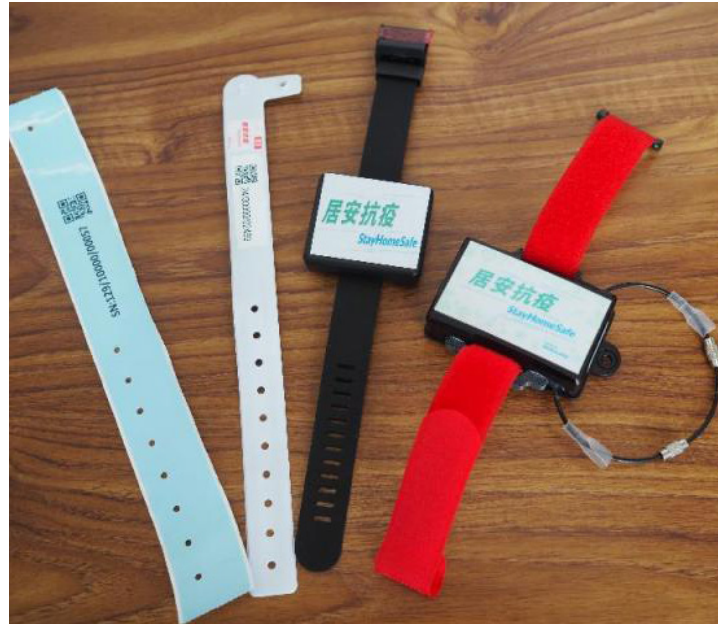
The BLE wristbands, which passengers arriving in Hong Kong must wear for the 14-day quarantine period (Image: Office of the Government Chief Information Officer)
