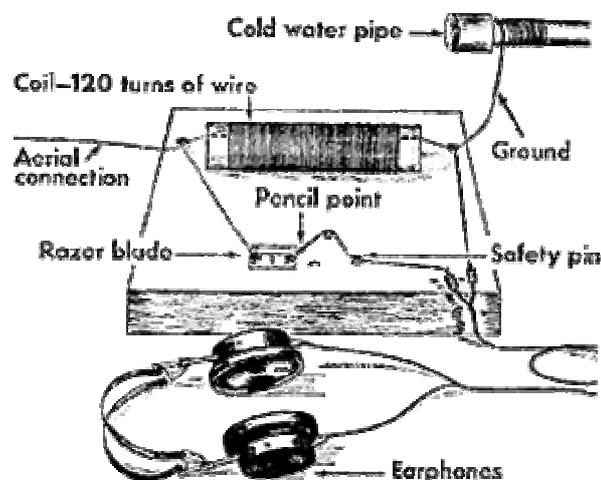
I have recently come across a sketch of a set that looked exactly like set 2 on the [Crystal radio page](#), except it had a razorblade/pencil detector where the diode would have gone.
