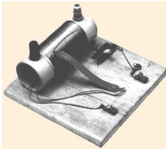
The photograph shows a similar radio built by Don Menning; he simply stuck the whole tip of a pencil on the end of the safety pin.
