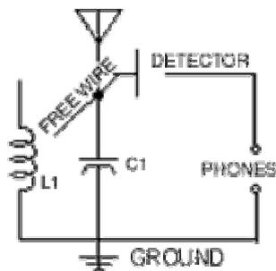
The simplest of these wartime sets didn't include a slider/tuner arm, and were therefore capable of only tuning in one frequency. An article appeared in a 1944 issue of QST, and is faithfully reproduced in the [D J Adamson Collection](#) pages, so I won't go into a lot of detail here except to include the schematic. I highly recommend visiting Mr. Adamson's pages if you are interested in old radio (or stereography).
