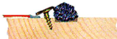
Remove the insulation from the ends of the wires coming from the coil, as well as from the ends of all wires used to make connections. Hammer a nail just to the left of the coil. Leave it sticking up just a bit. Wrap the bare wire from the end of the coil around this nail.
