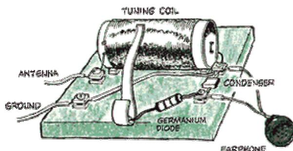
A-Dry a cardboard mailing tube in the oven, then paint with a coat of shellac. The tube should be about 6 or 7 inches long and 2 1/2 inches in diameter. Buy one pound of 26-gage (B. & S.) single cotton covered wire. Start and finish winding one half inch from ends of tube. Then shellac all over again. When dry, fasten down to a baseboard at each end, with a screw and washer to prevent it from touching at any point.
