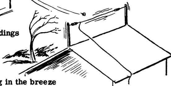
Signal losses will also be increased if a high resistance is present in the antenna circuit. To reduce resistance, all joints and connections should be carefully soldered and, wherever possible, the antenna and lead-in should consist of a single piece of wire with no joints.
