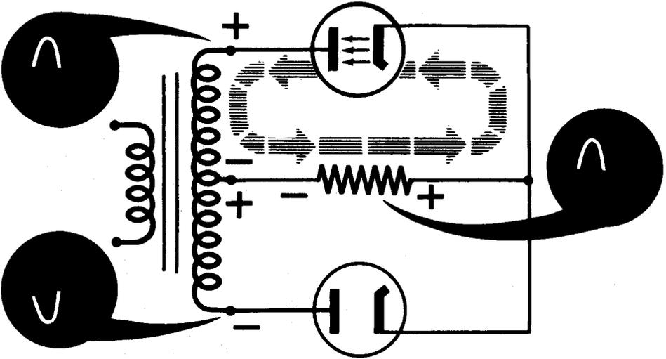
On the second half-cycle the plate of the upper diode is negative so that it cannot conduct, whereas the plate of the lower diode is positive so that current flows through it and through the load. Since both pulses of current through the load are in the same direction, a pulsating DC voltage now appears across the load. The full-wave rectifier has changed both halves of the AC input into a pulsating DC output.
