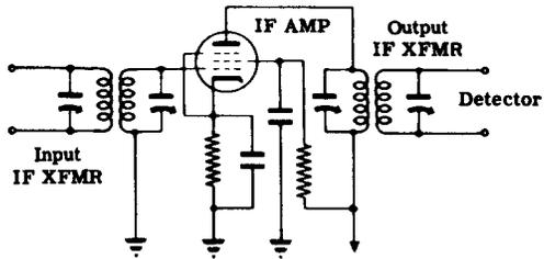
**DETECTOR AND AF AMPLIFIER**—These circuits perform the same functions as in the TRF receivers. In the superhet the diode detector is often combined with the first AF amplifier stage.
