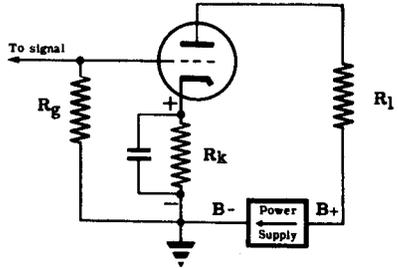
**TRIODE AMPLIFIER OPERATION** — The variation in voltage output (plate voltage) of a triode, used as an amplifier, may be ten or more times larger than the variation in the grid voltage (AC signal).
