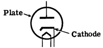
**ELECTRON EMISSION** — The action of the cathode in giving up electrons when the cathode is heated.
