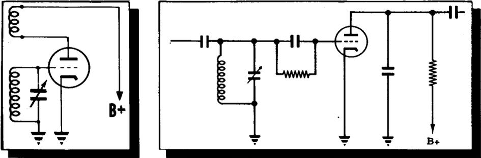
*An Oscillator + A Grid-Leak Detector*
