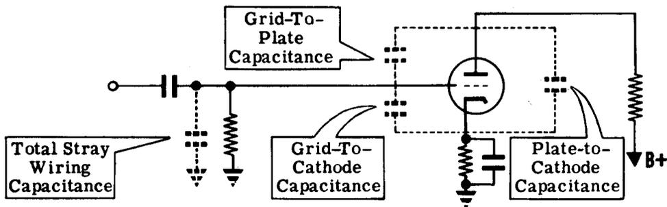
The effect of this total capacitance is to shunt the grid leak resistor. At low and medium frequencies the reactance of this small capacitance is high and therefore it does not disturb the operation of the circuit. At high frequencies, the reactance drops and effectively decreases the impedance between grid and ground. The signal appearing between grid and ground decreases as the impedance between grid and ground decreases.
