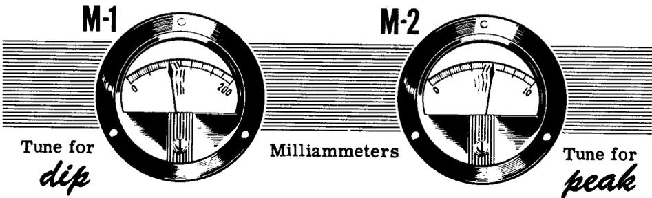
If the grid circuit has fixed bias or combination bias, no grid current will be drawn until the signal is fairly large. This will happen some time after the plate current meter has started to dip. For this reason, the rising grid current indication is sharper than the decreasing plate current indication.
