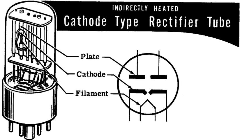
Vacuum tubes are constructed with a plug-in base which fits into a socket. The socket is permanently wired into the circuit and the tube is removable and easily replaced. Vacuum tubes have a relatively short life as compared to other components used in electronic equipment and a method of easy replacement is required.
