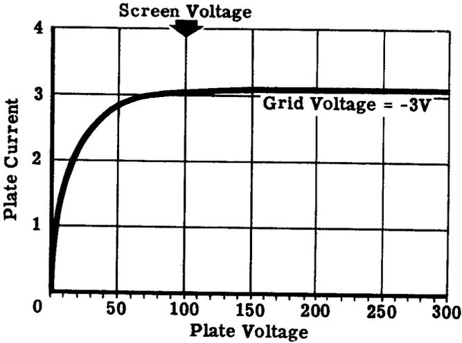
Curve No. 1: Over a wide range of plate voltages, the pentode plate current does not vary. But this is not saturation; in the next curve you will see that it is possible to draw more current than this. The reason the current doesn't vary over this range of values is that the screen shields the plate from the cathode's space charge.
