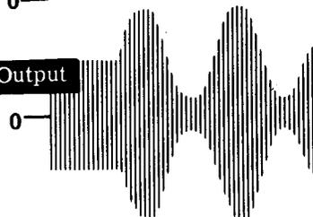
Grid modulation is used in compact or mobile transmitters because this type of modulation does not require a modulator with a large power output. When the modulator's weight is only a minor consideration, plate modulation with the larger modulator it requires is used because it produces much better results than grid modulation.
