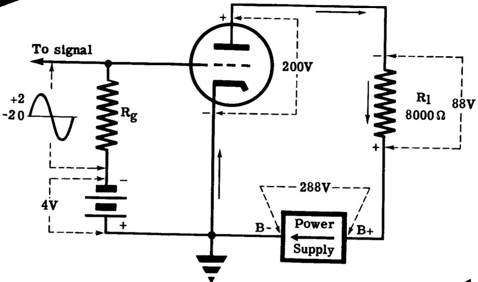
On the next sheet you will see how the load voltage and the plate voltage change when the signal is applied to the grid.
