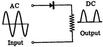
**RECTIFIER TUBE** — A vacuum tube diode consisting of plate and cathode which allow electron flow only from cathode to plate and thus acts as a rectifier.
