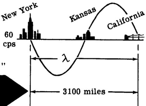
Similarly the wavelength of any frequency radiation can be determined by multiplying the constant velocity by the time for one cycle. Since the time for one cycle is equal to 1 divided by the frequency ( $\frac{1}{f}$ ), the wavelength equals constant velocity over frequency ( $\lambda = \frac{V}{f}$ ) or the velocity equals the frequency times the wavelength ( $V = f\lambda$ ). Since  $V$  is constant, the higher the frequency, the lower the wavelength and vice versa.
