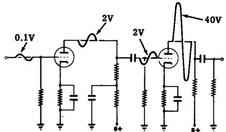
**AMPLIFICATION LOSSES** — At low frequencies the high reactance of the coupling capacitor reduces voltage gain; at high frequencies stray capacitance causes loss of voltage gain.
