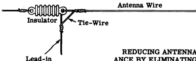
REDUCING ANTENNA RESISTANCE BY ELIMINATING JOINTS
