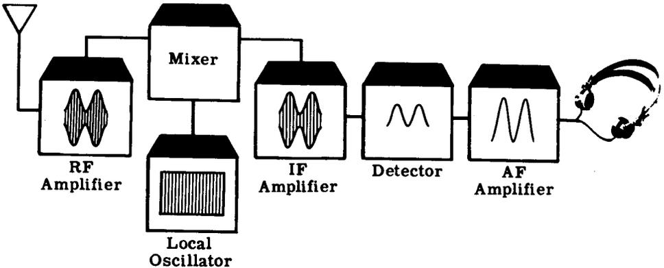
The process of mixing or beating two frequencies together to get a difference frequency is called "heterodyning." That is why the receiver was named superheterodyne.
