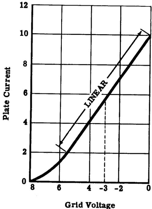
Curve No. 2: Here, you see that the control grid in a pentode controls current in the same way as it did in a triode. Normal grid bias for this particular pentode is about -3 volts.
