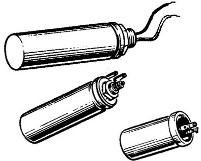
**WET ELECTROLYTIC CAPACITOR** — A condenser consisting of a metal electrode immersed in an electrolytic solution. The electrode and solution are the two condenser plates while an oxide film formed on the electrode is the dielectric. The dielectric film is formed by current flow from the electrolyte to the electrode.
