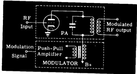
While the applied plate voltage is varying, a constant amplitude of RF is being fed to the grid of the tube from the output of the previous stage, the IPA.
