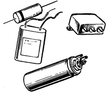
**PAPER FILTER CAPACITORS** — Paper filter condensers are bulky and their value is usually limited to less than 10 mfd. They are not polarized and can be made to withstand very high voltages. There is no appreciable leakage across a paper filter condenser. Oil-impregnated paper condensers are used in high voltage filter circuits.
