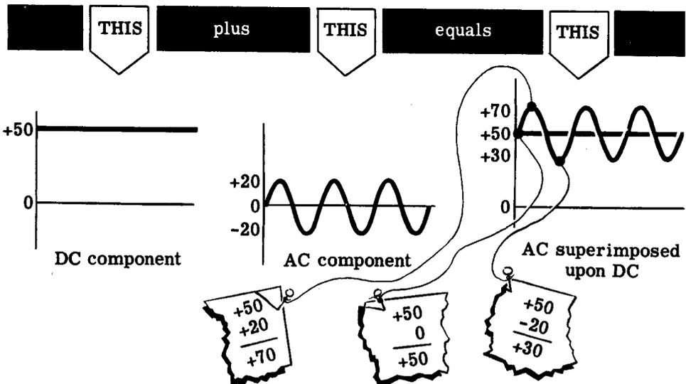
When the +20 volt AC peak is added to the +50 volts DC, the result is +70 volts. When the 0 volt point on the AC wave is added to the +50 volts DC, the result is +50 volts. When the -20 volts AC peak is added to the +50 volts, the result is +30 volts. The total result is a DC voltage which varies from +50 volts—up to +70 volts and down to +30 volts. The voltage of the resulting wave never becomes negative and yet it consists of an AC component and a DC component.
