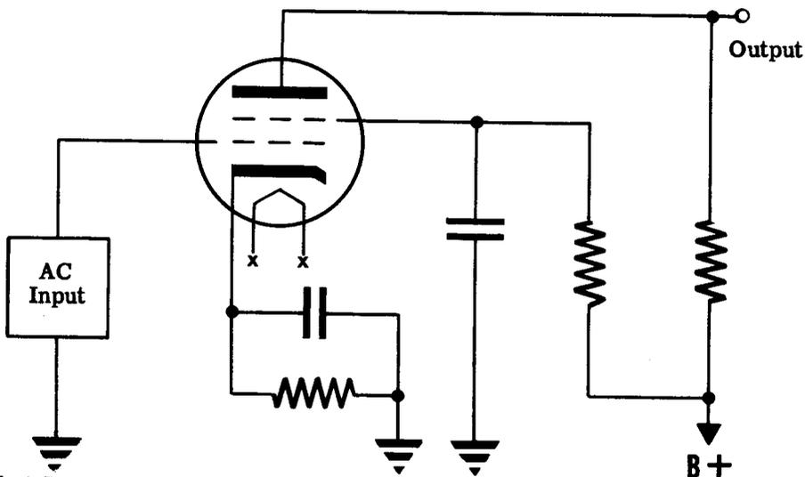
With AC on the control grid of the tube, the plate voltage will vary because of the drop in the load resistor just as in the triode. When the tetrode is used for getting large amplifications, the plate voltage varies over a wide range and, if it drops below the screen grid voltage, secondary emission effects cause distortion in the output.
