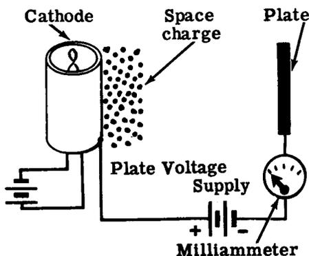
When the plate and cathode are at the same potential, the plate neither attracts nor repels electrons — the current is still zero.
