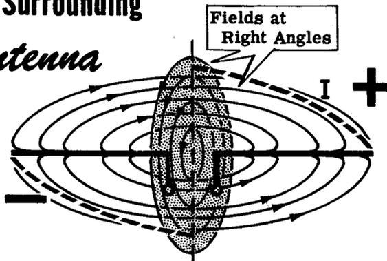
These electric and magnetic fields alternate about the antenna, building up, reaching a peak, collapsing, and building up again in the opposite direction, at the same frequency as the antenna current. In the process of building up and collapsing, a portion of these fields escape from the antenna and become the electromagnetic waves which radiate through space conveying the transmitted intelligence to distant receivers.
