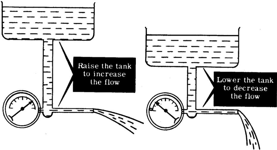
A much more convenient way to vary the flow of water is by using a faucet or valve in the system. Then, by simply turning the faucet, you can control the flow of water. Notice that the water pressure doesn't have to change in order to affect the flow.
