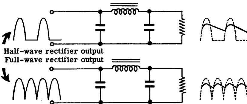
The higher the frequency of the AC input voltage to a power supply the lower the value of the filter condensers required. The time between pulses is shorter at higher frequencies and the inductive action of the choke is greater at higher frequencies.
