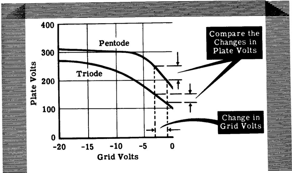
With a larger load resistor in the pentode circuit, larger amplification is obtained. This happens because the grid voltage, and only the grid voltage, can produce a change of current. This current will flow through the load resistor—the larger the resistor, the larger the voltage change.
