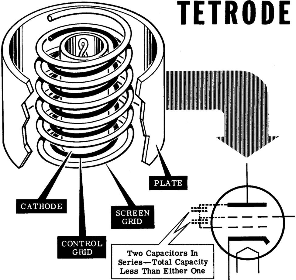
The plate is usually kept at a higher voltage than the screen and the plate circuit does not differ much from that which is used with triodes. In the tetrode, however, the plate voltage has less effect on the tube current than it did in the triode.
