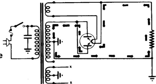
**HIGH VOLTAGE MEASUREMENT** — Always use only one hand in measuring voltages or testing circuits where high voltage is present. Use a test prod which is insulated and rated for working with high voltages.
