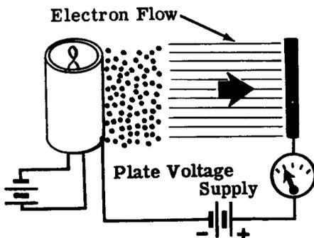
If this plate voltage is doubled, the current which flows is also doubled. This is the normal way for a diode to work: as long as the plate is positive with respect to the cathode, every change in plate voltage causes a corresponding change in plate current.
