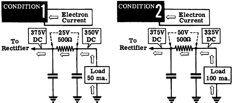
Similarly a change of 100 ma. in the load current will cause the B+ voltage to drop 50 volts. Such a rise and fall in output voltage is very undesirable in electronic equipment. Voltage regulator circuits might be added to compensate for this voltage change due to the filter resistor, but it would require a large and expensive circuit to compensate for changes such as are indicated here.
