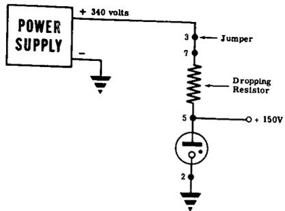
**VR TUBE JUMPER** — The purpose of the jumper in a VR tube is to prevent unregulated voltage from reaching a special electronic circuit if the VR tube is pulled out. Without the jumper, unregulated voltage would reach the circuit, causing improper operation and possible damage. Pulling out the VR tube removes the jumper and disconnects the voltage from the special circuit.
