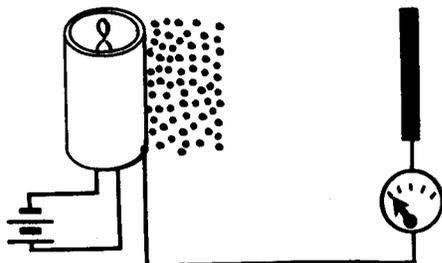
As soon as the plate becomes positive with respect to the cathode, current will flow from the space charge.
