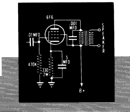
The 0.01-mfd coupling capacitor and 470K grid resistor found in the control grid circuit couple the control grid of the amplifier to the preceding detector stage. The capacitor also reduces the possibility that any DC voltages from the detector stage might be impressed upon the control grid of the amplifier.
