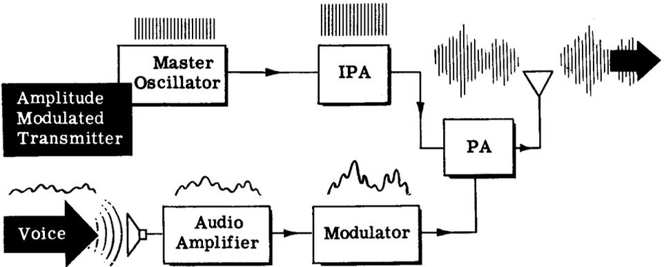
In the operation of an AM transmitter, it is essential that the modulator unit be on during transmission because the intelligence that is to be transmitted must come through the modulator. If the modulator is either off or defective, only unmodulated RF will be transmitted and a receiver at some distant point will not receive any message.
