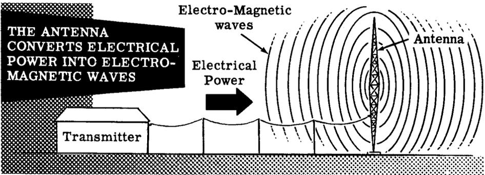
An interesting example of antenna action can be observed by touching your finger to the vertical input terminal of an oscilloscope. You will see a 60 cycle wave form on the 'scope screen which obviously must come from your body. What is actually happening is that your body is picking up 60 cycle electromagnetic waves which are radiated from the many power wires that carry 60 cycle current. The power lines are acting as transmitting antennas although they were not designed for that purpose.
