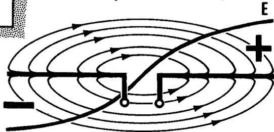
Besides this electric field, there is also a magnetic field which is generated by the antenna current. The plane of this magnetic field is at right angles to the direction of the current flow and therefore is at right angles to the antenna, as shown. The electric and magnetic fields must therefore be at right angles to each other.
