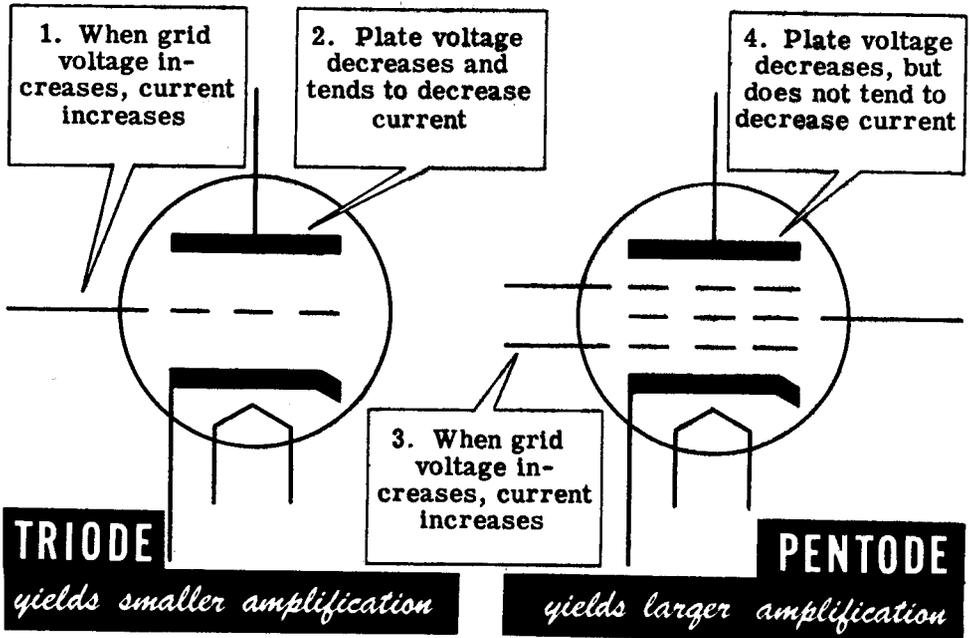
In the pentode the plate voltage can vary considerably with almost no effect on the current and, therefore, with no cancellation of the grid's control of the plate current. As a result, the amplification of a pentode is many times greater than that of a triode.
