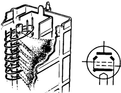
**PENTODE CIRCUIT** — A circuit providing proper operating voltages for control grid, screen grid and suppressor grid.
