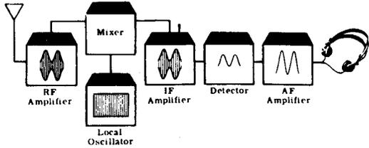
**MIXER**—This is the key circuit in a superhet. It takes the RF signal and beats it against the signal generated by a local oscillator. The resultant constant frequency signal is lower in frequency than the RF and thus is easier to amplify.
