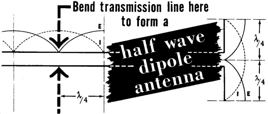
**RADIATION** — The voltage and current distributions along the antenna generate electric and magnetic fields at right angles to each other which are radiated into space as electromagnetic waves. These waves contain the intelligence of the modulating signal and can be detected by distant receivers.
