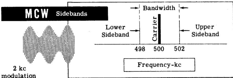
In a voice transmission, the modulating signal contains many frequencies—some as high as 5000 cycles per second. As a result, voice transmissions contain many sidebands (one sideband for each frequency) which may be as much as 5 kc above and 5 kc below the carrier frequency. This type of transmission, therefore, may cover a range of frequencies 10 kc wide.
