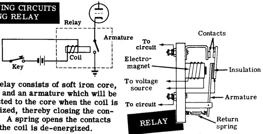
The relay consists of soft iron core, a coil and an armature which will be attracted to the core when the coil is energized, thereby closing the contacts. A spring opens the contacts when the coil is de-energized.
