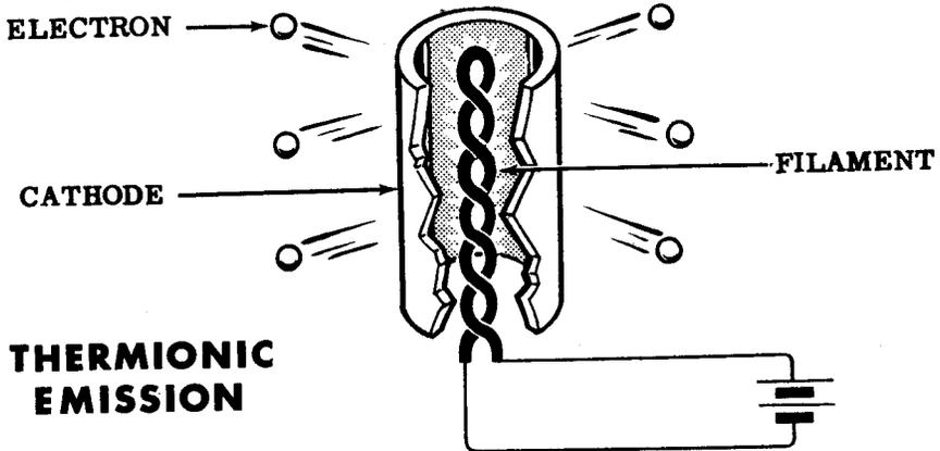
Some tubes such as the Fleming's Valve or the type 80 rectifier tube have what is known as directly heated cathodes, which means that there is no sleeve around the filament and the filament is itself the electron emitter.
