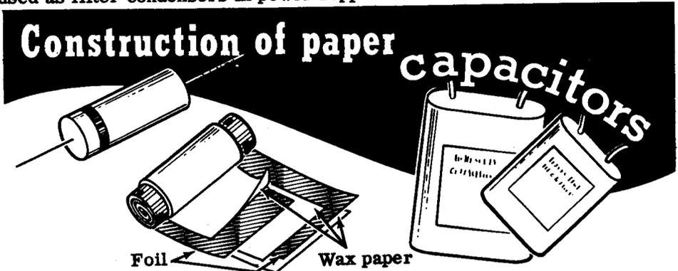
Paper condensers are not polarized and when operated within their voltage rating they last much longer than electrolytic condensers. However, large sizes of paper condensers are bulky and relatively expensive. They are normally not made larger than 16 mfd.
