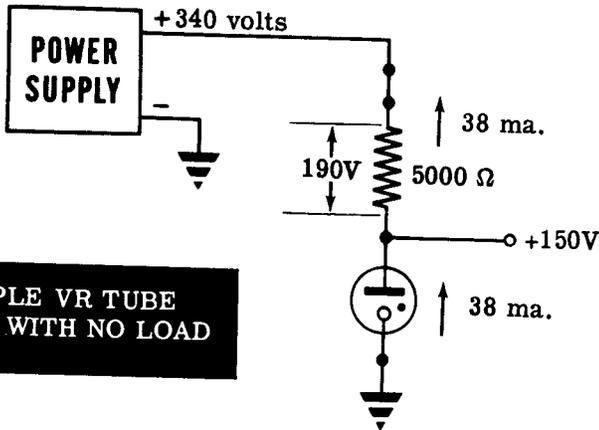
Suppose you attach an 8 ma. load to the 150 volt terminal. Of the 38 ma. flowing through the dropping resistor, 8 ma. flows through the load and 30 ma. flows through the VR tube. Since the VR tube current is yet within the rated range of 5 to 40 ma., the VR tube adjusts its internal resistance so that the plate voltage remains at 150 volts.
