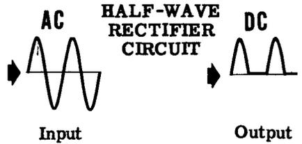
**DRY METAL RECTIFIERS** — A rectifier consisting of two unlike metallic substances pressed together, which allows current flow in one direction only. Copper-oxide and iron-selenium combinations are usually used to construct dry metal rectifiers.
