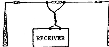
**LOOP ANTENNA**—The loop antenna is used with many portable and home broadcast-band receivers. Because it is highly directional, it is also used in direction-finding equipment.
