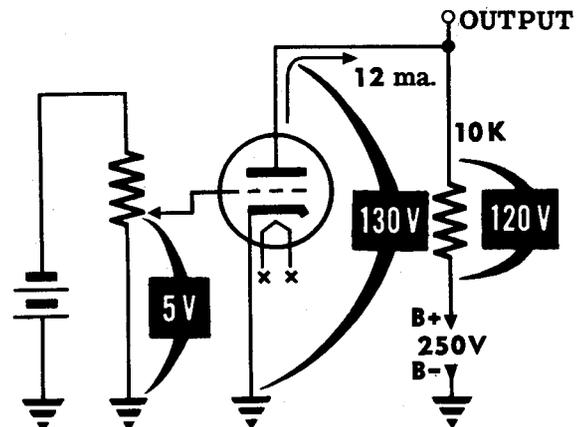
Now let's change the grid voltage from -10 volts to -5 volts (less negative). The current increases to about 12 ma., the drop across the load is 120 volts—an increase of 70V, and the voltage on the plate is now only 130 volts—a decrease of 70V. Note that the sum of these two voltages still adds up to the B+ voltage of 250V. Thus, a change of only 5 volts on the grid has changed the plate voltage 70 volts—an amplification of 14 times.
