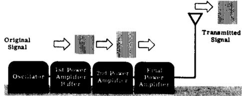
**TUNING METHODS**—The plate circuit of each transmitter stage may be tuned by adjusting the variable capacitor for minimum DC plate current.
