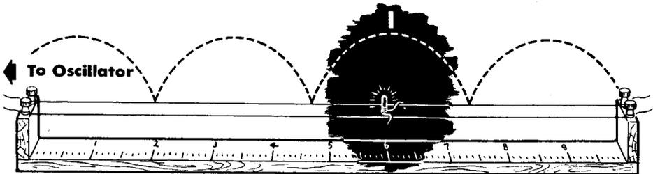
The voltage peaks can be found by using a neon bulb. The instructor holds the glass end of the bulb with his fingers and moves it along one wire, keeping a wire from the bulb in contact with the line at all times. The bulb remains out at the current peaks previously noted, but lights up between the current peaks, reaching maximum brilliance equidistant between two current peaks. The point of maximum brilliance is a voltage peak.
