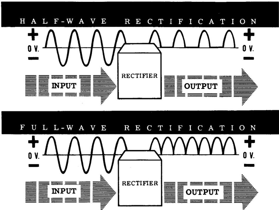
Notice that the DC output is not a constant voltage but rises and falls in time with the AC voltage input. When only the positive half cycles of the input voltage are allowed to pass through the rectifier and the negative half cycles cannot pass through at all, the process is called "half-wave rectification."
