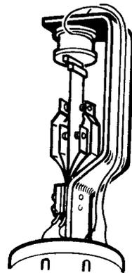
The two vibrating reeds shown connected together by the dotted line in the diagram are actually one reed placed between two pairs of contacts. The action of the reed between the transformer secondary contacts produces the same results as a full-wave rectifier. RF chokes and buffer condensers are used in this vibrator circuit in the same manner as in the non-synchronous vibrator to eliminate contact sparking and radio interference.
