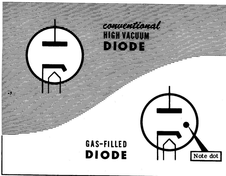
As you can see in the illustration, a gas tube has the same basic type of heater and cathode arrangement as the conventional diode. Many gas tubes have directly heated cathodes similar to the one in the type 80 high vacuum rectifier diode. Furthermore, the purpose of the cathode is the same in both types of tubes—to emit electrons.
