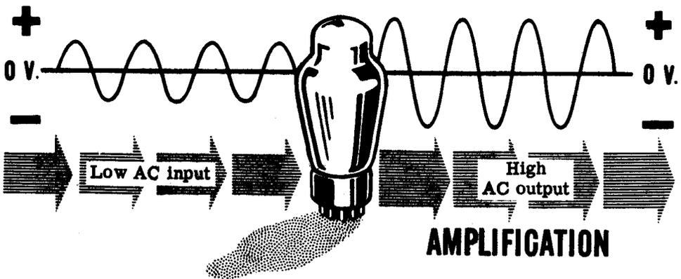
Because of your work with rectifier and power supply circuits, you now know all you need to know about rectification and the diode tubes that are used to do this job. Now you are ready to learn about the second main job a vacuum tube can do—amplification. In this section you will learn about the vacuum tubes that do the job of amplifying small AC voltages into large AC voltages.
