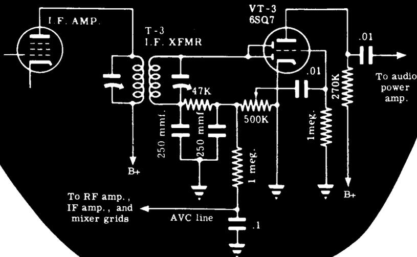
The two 250-mmf capacitors function as the detector filter capacitors. Their purpose is to bypass the IF component of the signal to ground around the 47K and 500K diode load resistors. The 47K resistor is part of the filter network, while the 500K potentiometer also acts as a bleeder resistor across the filter. It controls the amount of detector output delivered through the .01-mfd coupling capacitor to the grid of the first audio amplifier and thus serves as a volume control.
