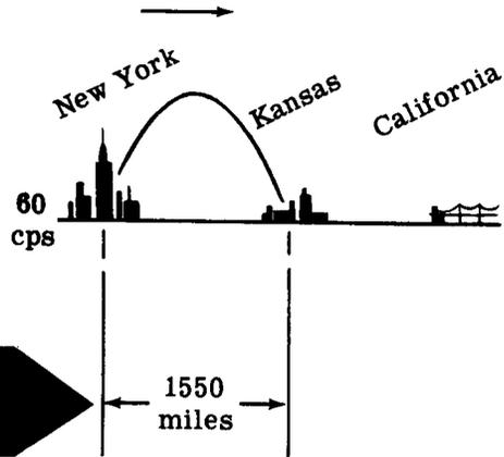
When another half cycle or a total of a full cycle has elapsed ( $\frac{1}{60}$  of a second), the zero voltage point will have traveled a distance of 3100 miles ( $186,000 \times \frac{1}{60}$ ) which is the approximate distance from New York to California. This distance of 3100 miles is the wavelength of the 60 cycle AC, which is the distance that the wave travels during the time interval for one cycle. The symbol for wavelength is the greek letter " $\lambda$ ".
