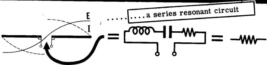
The radiation resistance is not an actual resistance. It is an equivalent resistance which, if connected in place of the antenna, would dissipate the same amount of power as the antenna radiates into space.
