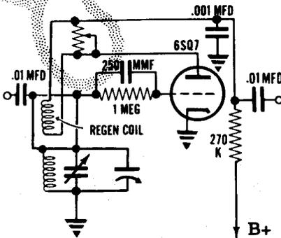
In the detector shown above, regeneration is controlled by a variable resistor placed across the tickler coil.
