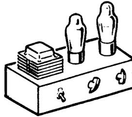
**HALF-WAVE RECTIFIER CIRCUIT** — A rectifier circuit using a single rectifier unit which changes AC to DC by allowing current to flow only in one direction. Alternate half-cycles of the AC power wave are utilized to provide a pulsating DC output. The circuit sometimes uses a transformer to increase or decrease the output voltage.
