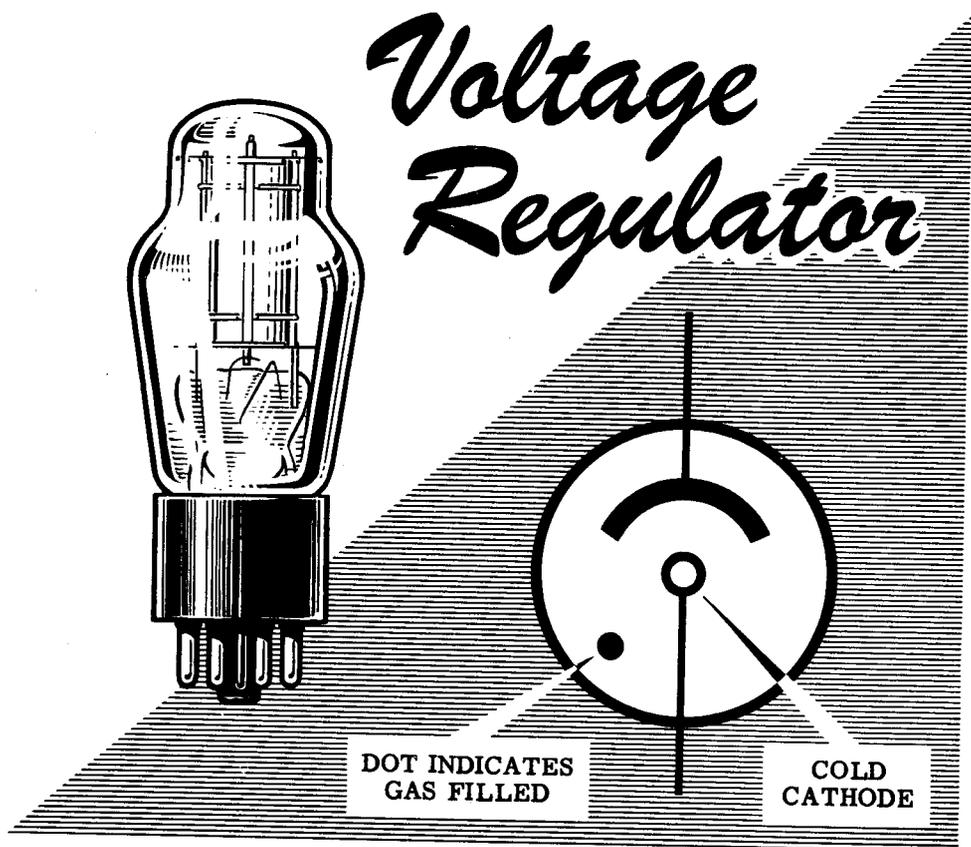
When a large enough potential is applied between the cathode and the plate, the gas in the tube conducts and electrons flow from cathode to plate. Conduction is characterized by a bluish glow inside the tube—the heavier the conduction the brighter the glow.
