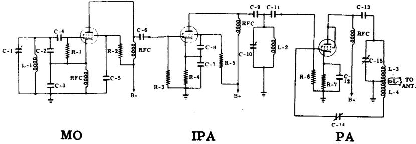
**TUNING**—For efficient operation, the plate tank circuit of the amplifiers must resonate at oscillator frequency. Adjusting the variable capacitor to reach this condition is called "tuning." Plate voltage is maximum and current minimum at signal frequency.
