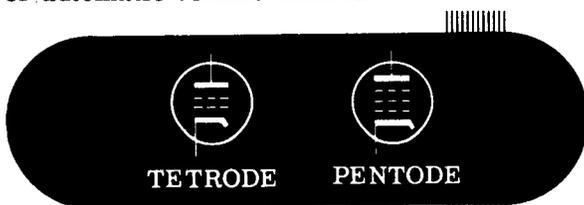
Only screen grid tubes are used in receiver RF amplifiers
