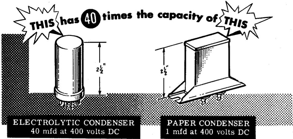
Power supplies rated at 600 volts or less usually use electrolytic filter condensers but when a higher voltage rating is required paper condensers are used. Electrolytics are polarized and failure to observe the correct polarity will not only permanently damage the condenser but may also cause it to break open and damage other parts.
