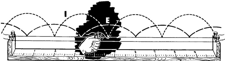
Both voltage and current peaks can be shown by using a long fluorescent light. The light areas are voltage peaks or current nulls.
