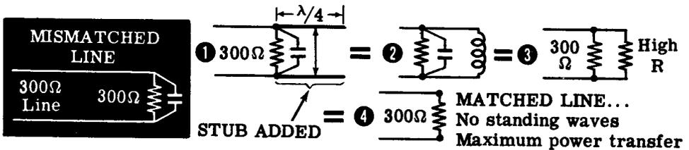
Quarter-wavelength sections are also used as transformers or matching devices to connect circuits of unequal impedances. If a low impedance input circuit is to be connected to a high impedance grid circuit, the input circuit may be tapped down on the coil of a tank circuit as shown. If a tuned line is used, the input circuit can similarly be tapped down on the tuned line. This is an example of a tuned line used as a step-up transformer.
