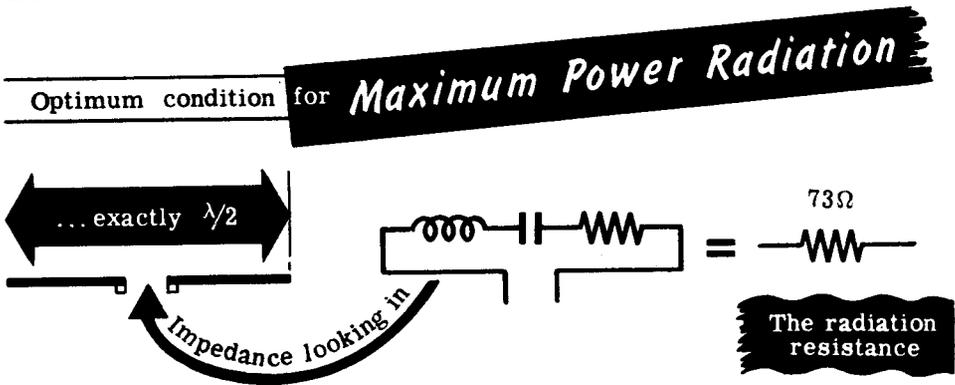
If the frequency of the transmitter goes up, the antenna will be longer than a half wavelength. The series circuit is then operating at a frequency which is above its resonant frequency. At this applied frequency, the inductive reactance is larger than the capacitive reactance and the antenna appears inductive to the transmitter.
