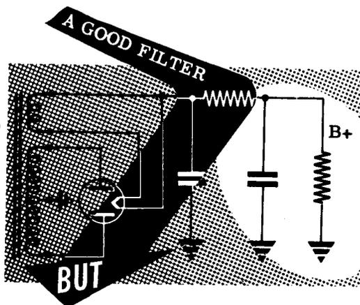
What the filter circuit requires is that the resistor have a high resistance for AC and a low resistance to DC. A resistor presents exactly the same resistance to both AC and DC and cannot meet this requirement. When a filter resistor is used, its size must be a compromise between these two opposing requirements.
