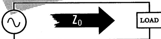
An example of getting maximum power transfer from a transmission line to a load is the case of a line feeding an antenna. If a certain type of antenna, called a "half-wave dipole," is used, the impedance at its center feed point is 73 ohms. Therefore in order to get maximum power transfer from the transmission line to the antenna, the characteristic impedance of the line should be 73 ohms or close to it. When this is the case, the line is said to be "matched" to the antenna.
