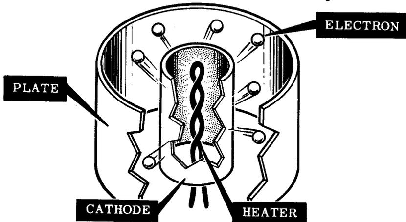
In addition to preventing the filament from burning, removing the air from the tube prevents the air molecules from interfering with the flow of electrons from cathode to plate. Sometimes the air is replaced by an inert gas which aids rather than opposes the electron flow.
