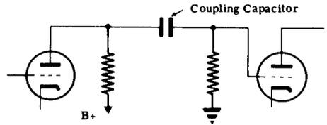
**VOLTAGE GAIN** — The total amplification of a two-stage (or multistage) amplifier is the product of the amplifications of each stage. The ratio of the output voltage of final stage to the input voltage of first stage is called the gain of the amplifier.
