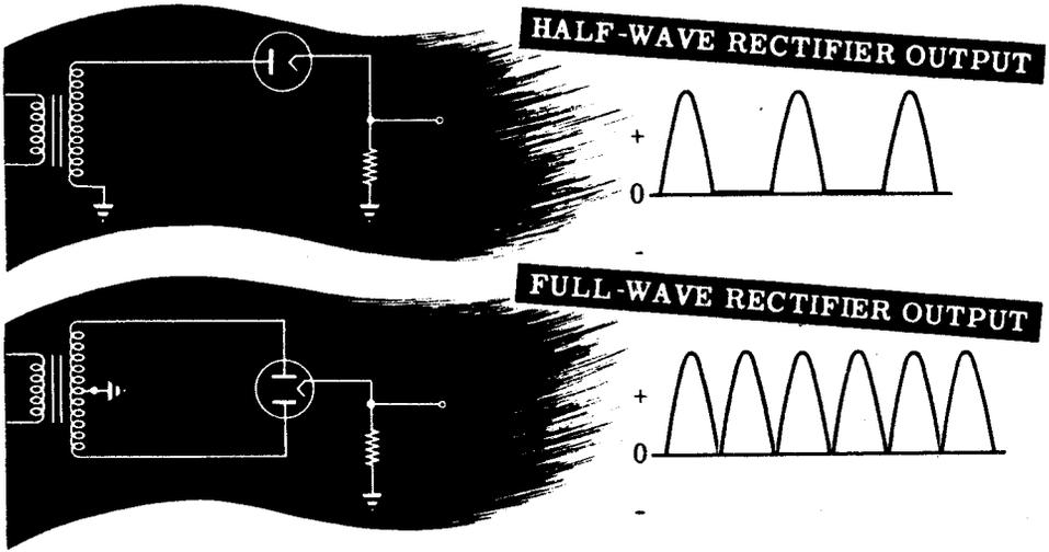
The electronic circuits which are connected to the power supply output cannot use a pulsating voltage of this sort. What these circuits require is a steady DC voltage with as little pulsation as possible. The purpose of the filter circuit is to remove the pulsations from the rectifier output and deliver a steady DC voltage.
