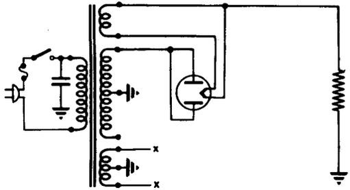
**CURRENT FLOW IN A HALF-WAVE RECTIFIER CIRCUIT** — AC is applied to the rectifier plate and current flows only during those half-cycles which are positive on the plate side of the circuit input.
