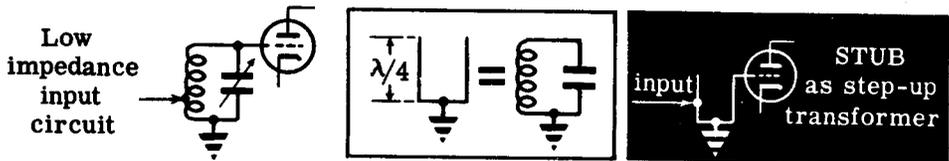
A quarter-wave stub can be used as a step-down transformer to match a high impedance line to a low impedance dipole antenna. The line is connected to the high impedance input of the stub and the antenna is connected near the low impedance shorted end of the stub.
