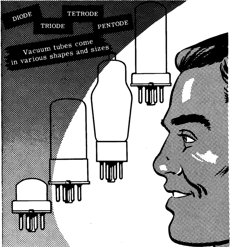
Their names describe them by telling how many parts (cathode, grid, plate) there are in the tube. A diode (di = two) has two parts—a cathode and a plate. A triode (tri = three) has three parts—a cathode, a plate and one grid. A tetrode (tetra = four) has four parts—a cathode, a plate and two grids. A pentode (penta = five) has five parts—a cathode, a plate and three grids.
