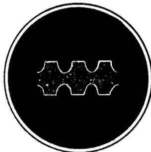
If the transmitter output shows breaks in the modulation pattern, the transmitter is said to be "over-modulated." This is usually due to excessive modulating voltage but may also be due to insufficient signal voltage on the grid or excessive grid bias voltage.
