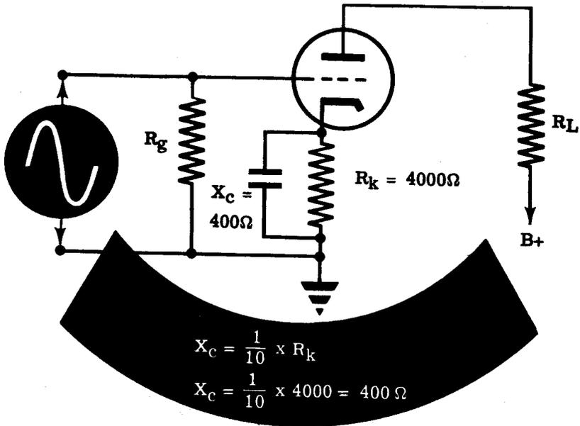
Since  $X_c = \frac{1}{2\pi fC}$ , the capacity of the bypass condenser can be found by using the formula  $C = \frac{1}{2\pi fX_c}$ , where  $f$  is the lowest frequency signal to be amplified. Suppose  $f$  is 60 cps and  $X_c$  is  $400\Omega$  as shown above, then  $C$  will be—
