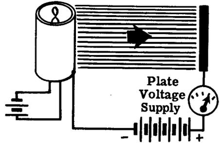
At this point, a further increase in plate voltage does not result in any additional current. The current does not increase because the cathode is emitting all the electrons it can. It is NOT normal to operate a diode at such a high plate voltage that changes in plate voltage do not produce changes in plate current.
