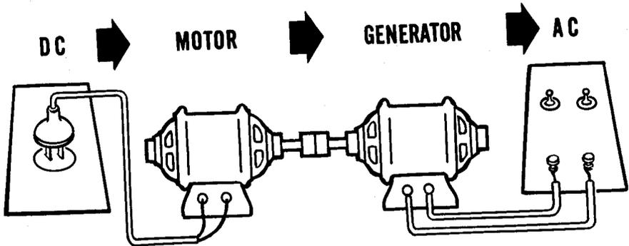
A dynamotor is a rotating DC machine that operates from a low voltage DC source and puts out one or several high voltage DC outputs. It is basically a DC motor and a DC generator built onto one armature and having two or more windings and two or more commutators. Dynamotors are usually operated from 6-, 12-, 24- or 32-volt storage batteries and deliver from 250 to over a thousand volts DC at various current ratings.
