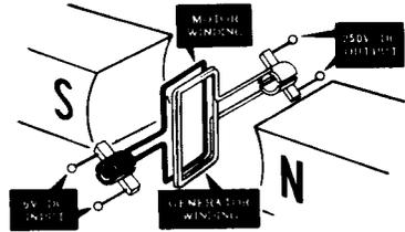
**ROTARY CONVERTER** — Rotary converters are commonly used to change AC to DC, but they may be used to operate from storage batteries to give an output of 117 volts AC and are then known as inverters. The construction of a rotary converter is similar to a DC generator except that two slip rings are used which are connected to commutator segments 180 degrees apart.
