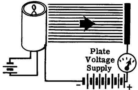
If we now increase the filament voltage above its normal value, we enable the cathode to emit more electrons and, with the same plate voltage as before, we observe that a larger plate current is flowing.
