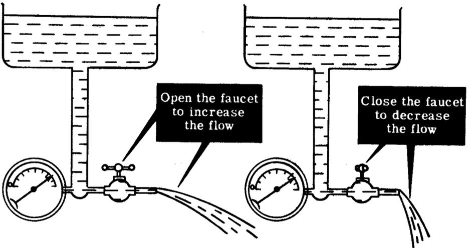
This is similar to the way a triode tube amplifies the flow of current. In the triode an additional element, the grid, is placed in the tube, its purpose being to control the flow of current in the tube just as the faucet controls the flow of water. You will see that a small voltage variation on this element produces a comparatively large current variation in the tube.
