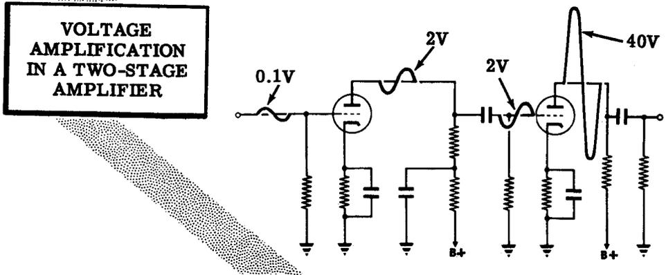
Suppose each amplifier stage can deliver an amplification of 20. If a 0.1 volt AC signal is applied to the grid of the first stage, the output of this stage will be  $20 \times 0.1 = 2\text{V}$ . Since the output of the first stage is connected to the input of the next stage there will be 2 volts AC on the grid of the second stage. The second stage amplifies the signal 20 times and produces an output voltage of  $20 \times 2 = 40\text{V}$ .
