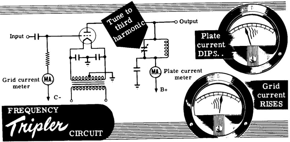
**FREQUENCY Tripler CIRCUIT**
