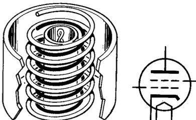
**THE PENTODE** — A tube which uses a suppressor grid between the screen grid and plate to reduce the effect of secondary emission. It has greater amplification than the triode.
