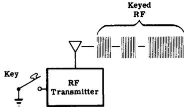
**MCW TRANSMISSION**—A constant amplitude audio frequency signal is superimposed on the RF carrier wave. Transmitter is turned on and off by means of a key as in CW transmission. MCW is used for emergency applications.
