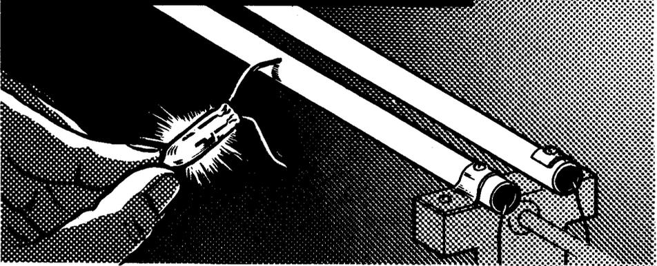
Once oscillations have been verified, the instructor demonstrates the presence of standing waves along the half-wave antenna by holding a fluorescent lamp close to and parallel with the antenna. The lamp is ignited by placing one end against the tuned line. The lamp glows at the ends and is out in the middle.
