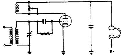
**PLATE DETECTOR**—This detector employs a triode or pentode, biased near cut-off. Rectification takes place in the plate circuit since the negative half of the modulated RF grid signal drives the tube into cut-off.
