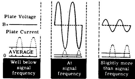
**NEUTRALIZATION**—Plate or grid neutralization circuits may be used to counteract the feedback effect at the grid-to-plate capacity of triodes used in transmitter amplifiers.
