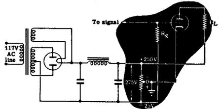
**CATHODE BIAS** — A cathode bias resistor in parallel with a cathode bypass capacitor in the cathode circuit provide the most widely used system of biasing.
