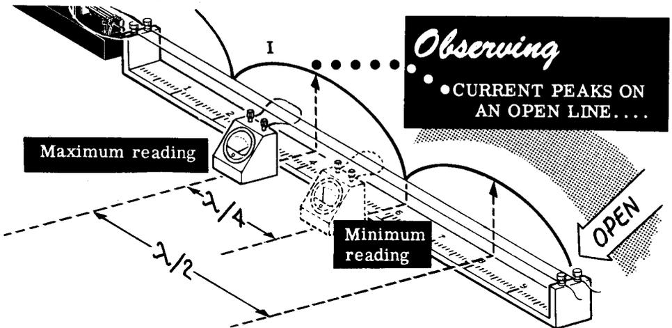
The meter indicator is placed at a point of maximum current, and the instructor shorts the open end of the line with a screwdriver. The reading drops immediately and the meter is moved to the new current peak which is a quarter wavelength away from the previous current peak position. The short has displaced the standing waves one-quarter wavelength from their position when the line was open. The short is removed and the demonstration continues.
