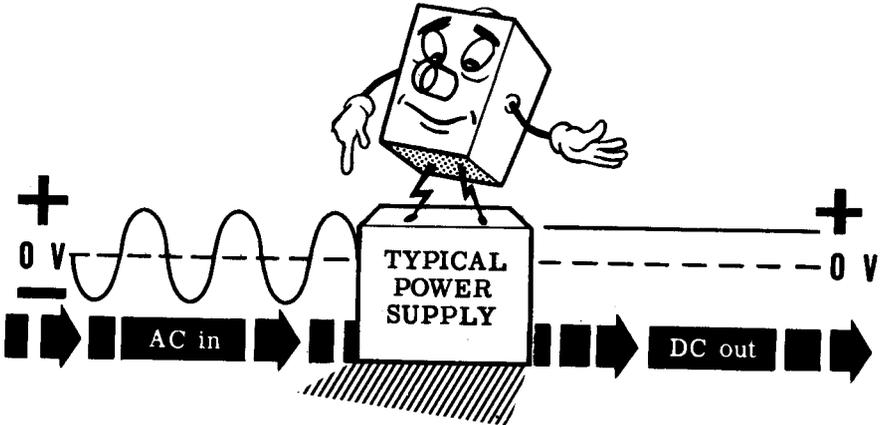
The reason why different types of power supplies are required is simple. One power supply you may build would go up in smoke if you drew much more than 150 ma. of current from the high DC voltage supply. Certain types of transmitters require as much as 5,000 or 10,000 ma. from their power supplies. Certain special oscilloscope circuits may require a DC output of 10,000 volts or more.
