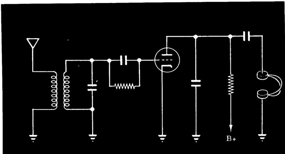
You will recall that the plate current of a triode is dependent upon the grid voltage. Consequently the audio frequency variations in bias should produce a corresponding pulsating plate current. Any radio frequency component of the plate current is filtered out by capacitors and RF chokes placed in the plate circuit. As a result, the voltage developed across the plate load is an amplified reproduction of the audio frequency voltage developed across the grid-leak resistor.
