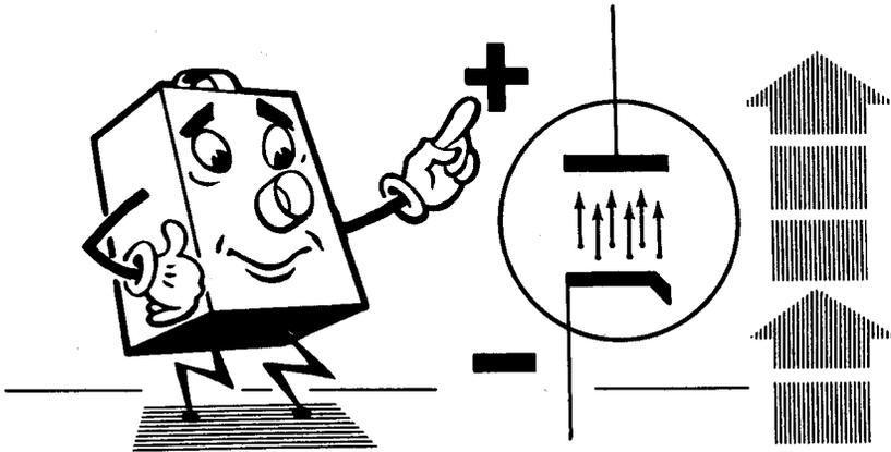
2. The diode does not allow electrons to flow through it when the plate is negative with respect to the cathode.
