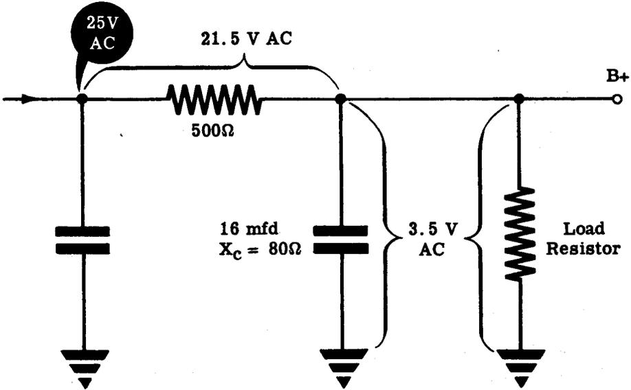
You see that the simple addition of a 500 ohm resistor and another filter condenser has succeeded in reducing the ripple voltage down to 3.5 volts which is about 1 percent of the total DC output. This amount of filtering is satisfactory for most applications in electronics.
