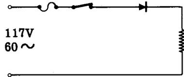
**RECTIFIER CIRCUIT WAVEFORMS** — If the applied voltage is an AC sine wave, the output waveform consists of half cycles of the applied AC voltage. This output waveform is a pulsating DC voltage.
