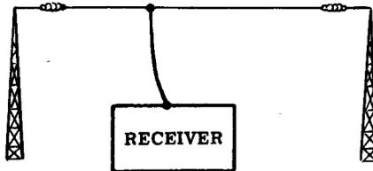
**DIPOLE ANTENNA**—This type of antenna is the same as is used in transmitters, and consists of two quarter wavelength sections supported horizontally. It gives excellent high-frequency response.
