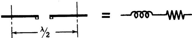
If the frequency of the transmitter goes down, the antenna will be slightly shorter than a half wavelength. The series circuit is then operating at a frequency which is below its resonant frequency. The capacitive reactance is larger than the inductive reactance and the antenna appears capacitive to the transmitter.
