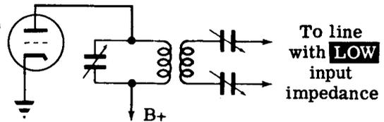
When a transmission line has a high input impedance, parallel tuning, called "voltage feed," is used. Here the high impedance of the parallel tank circuit matches the high input impedance of the line, and maximum power transfer is effected.
