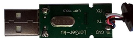
GND is Black, TX is Red, RX is White
