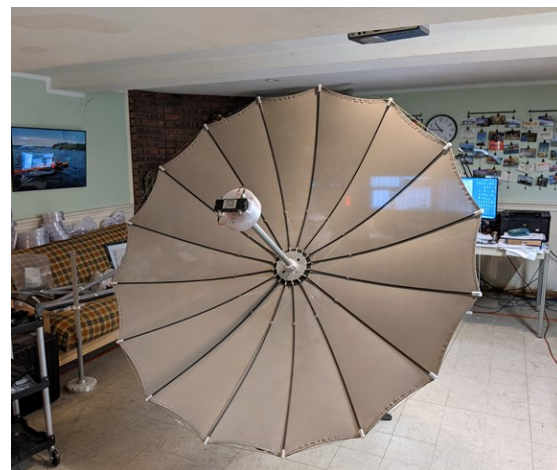
Figure 2 – New Antenna - Folding Parabolic Dish by W2HRO [1]
