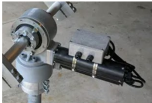
Figure 4 – DC-based Slew Drive High Accuracy Rotator
